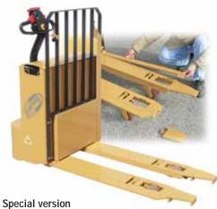
with lateral handle fasteners, including load backrest and, if required, detachable fork extensions.
